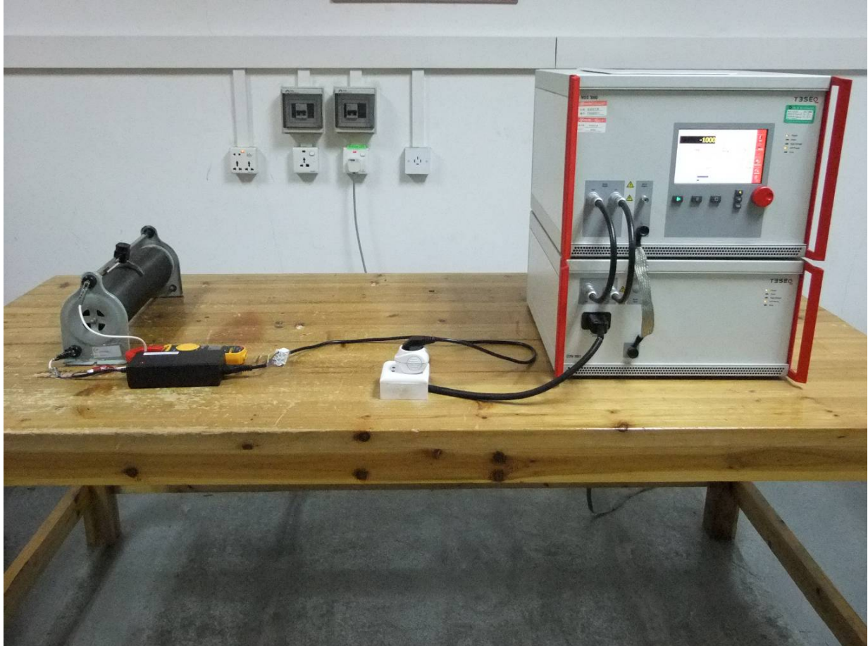
Photograph 6: Set-up for Surge on AC Power Supply
