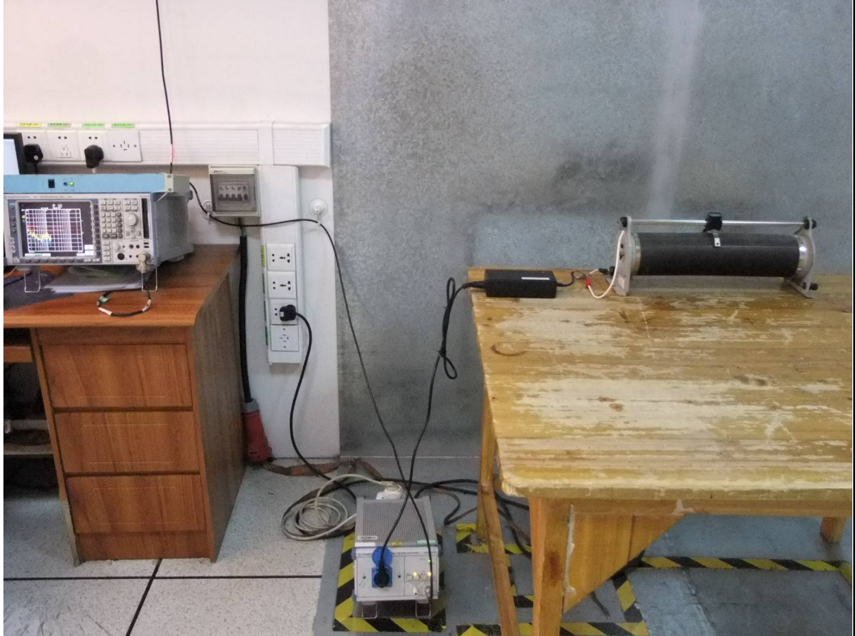
Photograph 2: Set-up for Terminal Continuous Disturbance Voltage on AC Mains
