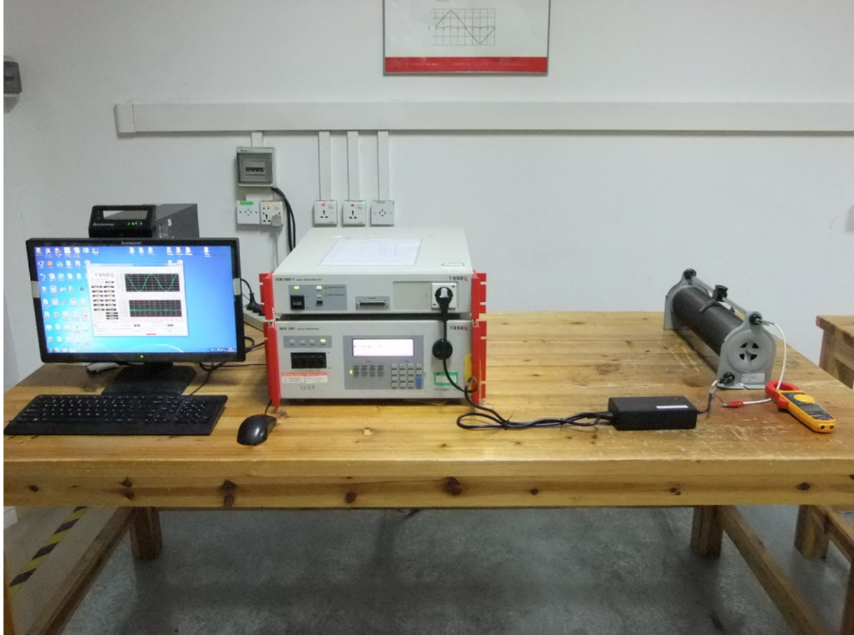
Photograph 1: Set-up for Harmonics Current Emission on AC Mains
