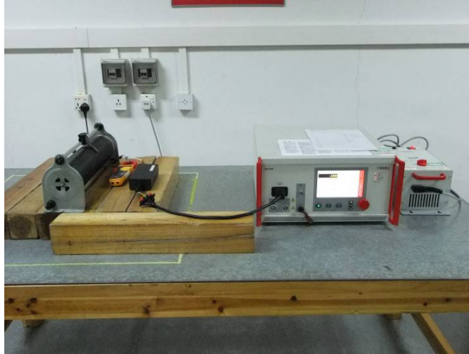
Photograph 5: Set-up for Electrical Fast Transient (EFT)
