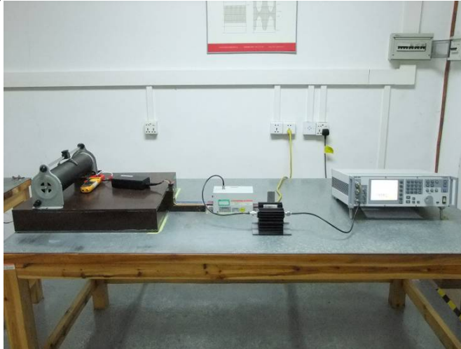
Photograph 4: Set-up for Radio-frequency Common Mode / Conducted Susceptibility (CS)
